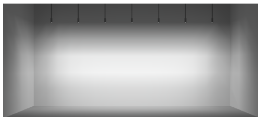
10FT CEILING 36" SETBACK / 48" ON CENTER SPACING
