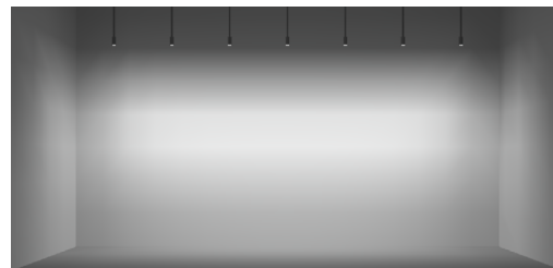
12FT CEILING 36" SETBACK / 48" ON CENTER SPACING
